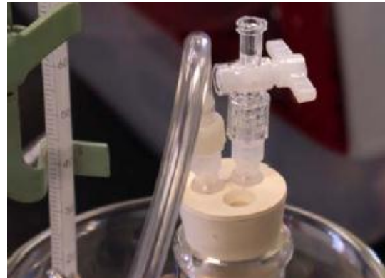
Figure 6. Closed to the atmosphere. Any gas generated in the tube will be contained and monitored by the pressure sensor.
