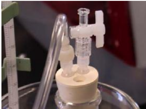
Figure 5. Open to the atmosphere. Any gas generated in the tube will be vented to the air
