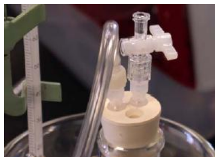
Figure 6. Closed to the atmosphere. Any gas generated in the tube will be contained and monitored by the pressure sensor.
