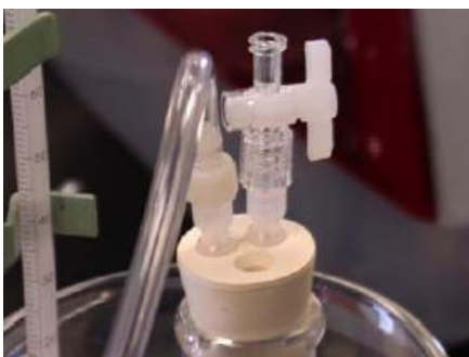
Figure 5. Open to the atmosphere. Any gas generated in the tube will be vented to the air
