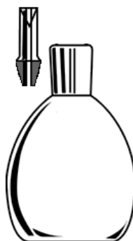
Figure 2. A sketch of a pycnometer and a one filled with a blue solution.
