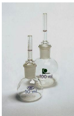
Figure 1. Pycnometers come in a variety of sizes. A 25 mL pycnometer will be used in this lab activity.
