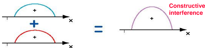
Figure 1. The combining of the electron waves of two hydrogen atoms that are in phase.
