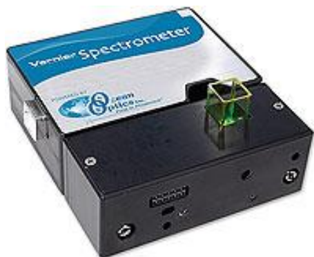
Figure 6. A Vernier spectrophotometer containing a cuvette containing a Nickel (II) sulfate solution.
