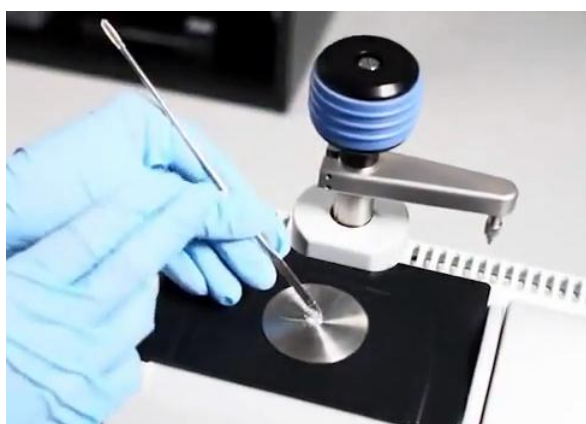
Figures 2 and 3. Place a solid sample on crystal surface and then press it against surface of crystal by turning down on knob. The tightening works the same way as a gasoline tank cap on an automobile—it begins “ratcheting” when it can be tightened no further.
