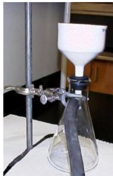
Figure 2. Büchner funnel set-up for suction filtration.
