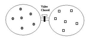
7a. Complete the drawing of the system once the stopcock is opened and the system reaches a material equilibrium.
