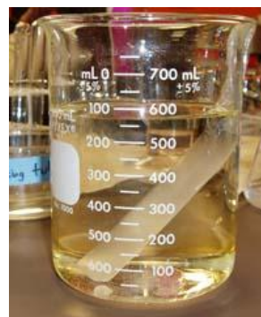
Figure 2. Set-up for the investigation of the permeability of dialysis tubing. A 400 mL beaker will be used in this experiment.
